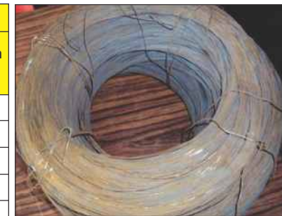
Local Binding Wires
